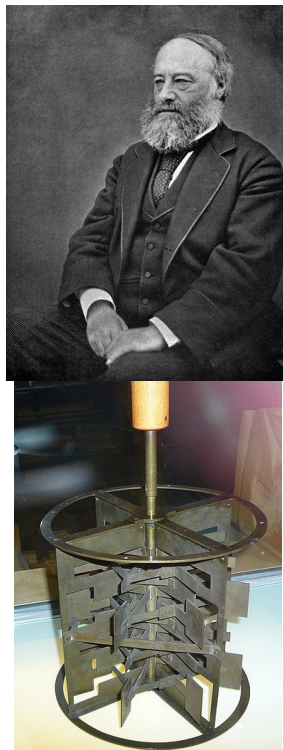
Figure 1. (left) James Prescott Joule (1818 - 1889) (right) Joule's apparatus for measuring the work equivalent of heat. (CC BY-SA 3.0; Dr. Mirko Junge)
